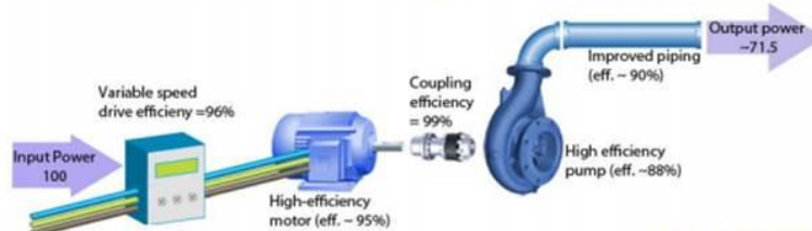
Efficiency Optimized Pumping System (Efficiency ~ 72%)
